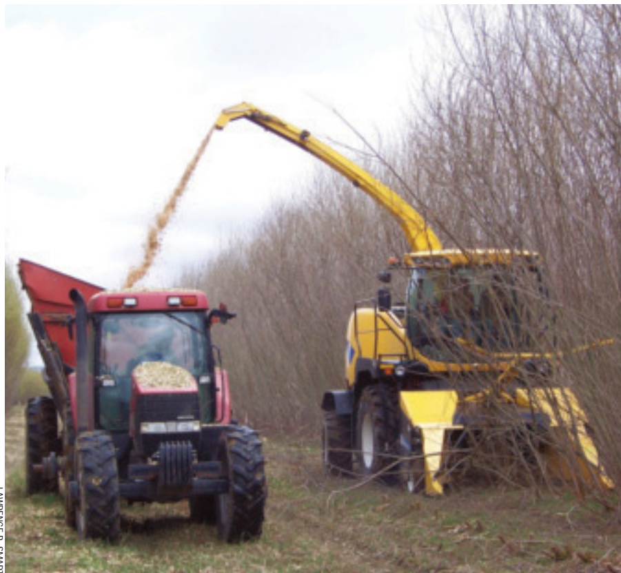
Spring willow harvesting with a New Holland FR series forage harvester outfitted with short-rotation woody crop cutting head.
