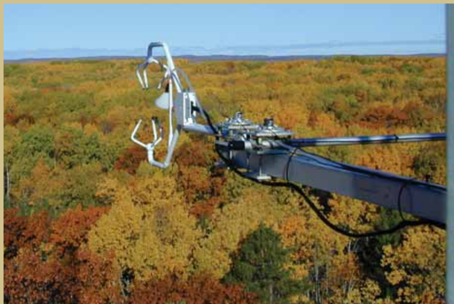
A sonic anemometer for monitoring gas exchange between the forest and the atmosphere.
